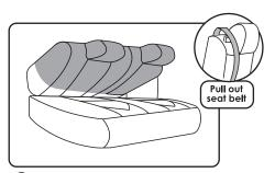
(3) For the backrest 60 side, split the seats and place the seat cover over the car seats. Note, make sure you pull out the seat belt.
