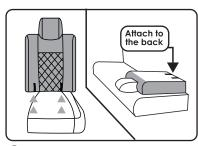
(2) For the backrest 40 side, pass the hook-and-loop straps which are indicated by the arrows through the cervice of the seat. We reccommend you split the car seat and attach it to the back of the seat as illustrated above.
