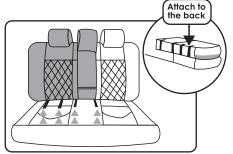
Push the rear hook-and-loop straps through the seat crevice. Attach the straps directly to the upholstery of the backseats.
