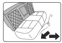
(5) Remove the bottom seats by pushing diagonally inward then pulling the bottom bench seat cushion up and out.
