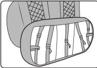
6 Place the bottom seat cover on the bench seat cushion and attach the buckles as shown above. Once complete, reattach the bottom bench seat cushion to the vehicle.
