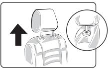
1 Detach the headrest by pressing the button located at the base of the headrest. Then simply lift the headrest to separate it from the backrest.
