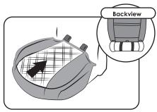
(a) To install the bottom cover, place it on the seat and push the buckle straps through the seat crevice. Then, pull them out from the backside of the seat as shown in the image above.
