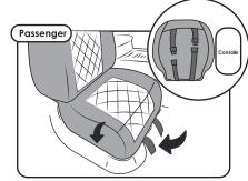
(a) Tuck in the bottom cover around the seat, especially next to the center console, to ensure a snug fit. Finally, attach the buckle straps underneath the seat. TIP: Use a plastic tool to tuck in the cover easily.
